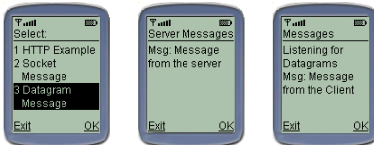
Figure 13.12 Running the MsgClient and MsgListener passing datagrams. The MsgListener waits for activity on a specified port. When a datagram is sent from the MsgClient , the MsgListener receives the datagram and responds appropriately.
