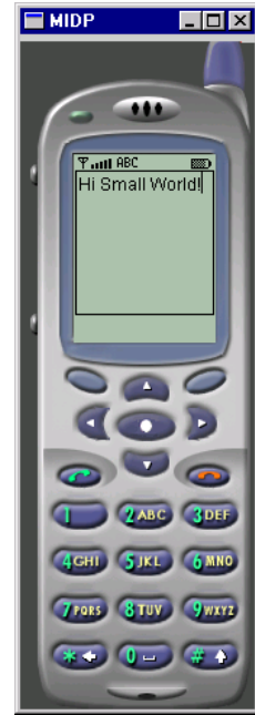
Figure 4.1 The HiSmallWorld MIDlet written above is depicted here running in the MIDP emulator. While the MIDP specification dictates common Java functionality across the spectrum of devices, in this case cellular telephones, each device may have a slightly different display. Thus, emulators often provide various “skins” to test applications running in various displays.
