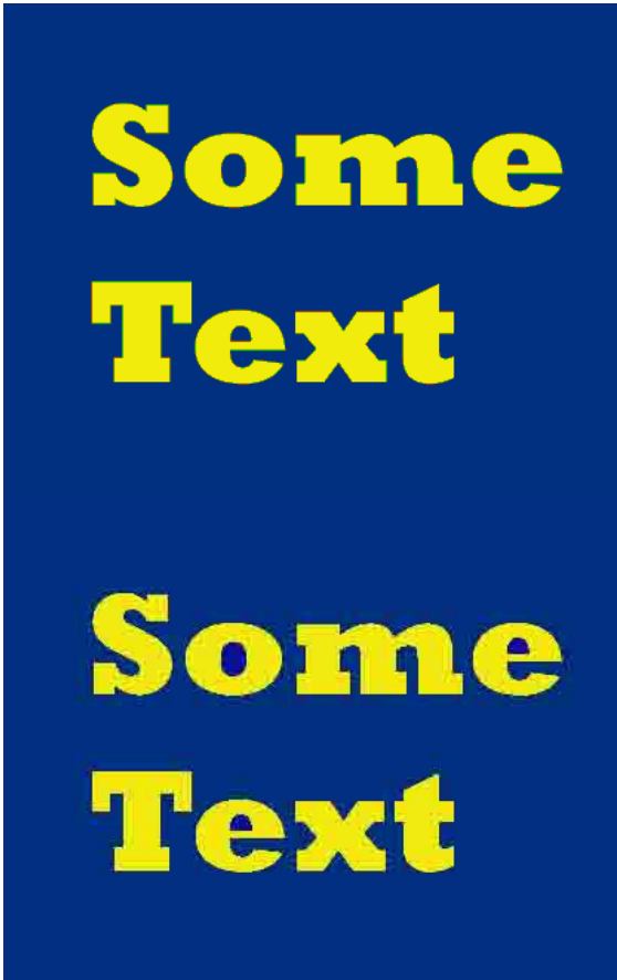
Figure 1.2 The result of lossy compression on a simple image. Notice the imperfections around the edges of the text in the second image.
