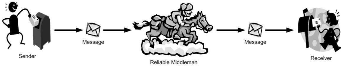
2 Figure 2.2: Java EE adds reliability to messaging by adding a reliable middleman that guarantees the delivery of messages despite network outages, even if the receiver is not present on the other end when the message is sent. In this sense, Java EE messaging has much more in common with the postal service than it does with common RPC protocols like RMI. We will discuss this model in much greater detail in Chapter 5.
