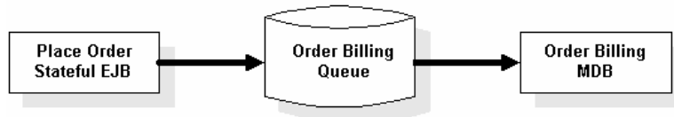
3 Figure 2.3: Asynchronously order billing using MDBs. The Stateful Session Bean processing the order sends a message to the order-billing queue. The billing MDB picks up this message and processes it asynchronously.
