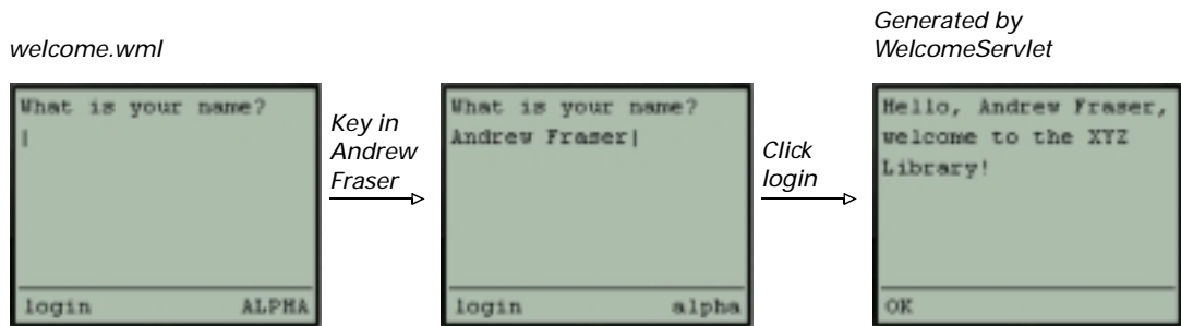
Figure 24.9 Passing name parameter to WelcomeServlet from welcome.wml using <go> and <postfield>
