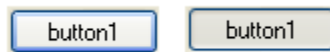
Figure 1.2 To have a control change state, you have to force it to redraw itself, as with these buttons shown pre-and-during a click.
