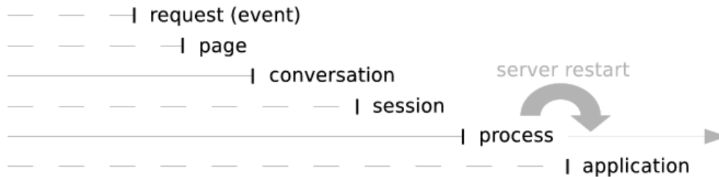
Figure 1.8 The lifetimes of the six scopes in a Seam application. The standard scopes are represented by dashed lines, while the scopes that Seam contributes are shown as solid lines. The business process scope is persisted to a database and can thus outlive the application scope when the application server restarts.
