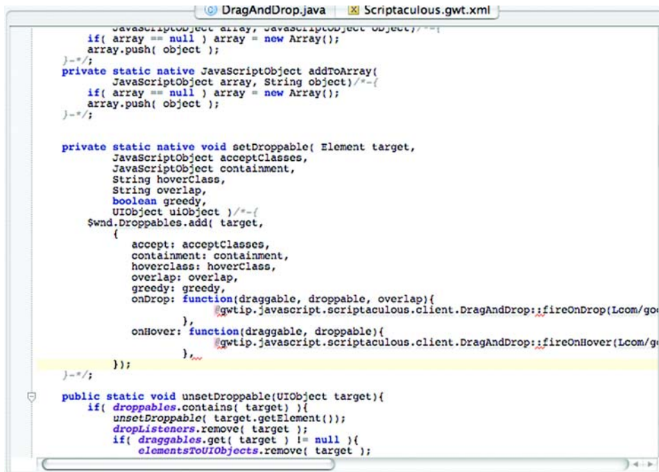
Figure 6.2 IDEA's syntax highlighting of the JavaScript inside the setDroppable() method. The JavaScript syntax highlighting of JSNI methods is one of IDEA's greatest GWT features.
