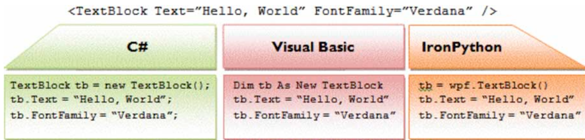
figure 1.6 Any object that we create in XAML can also be created within code.
