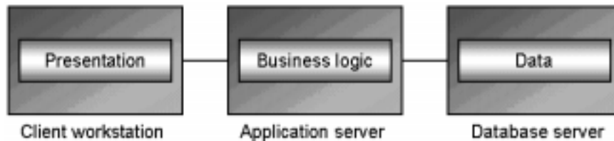
Figure 1.9 Three-tier application partitioning
