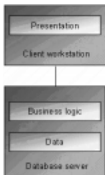
Figure 1.7 2 1/2-tier (fat server) architecture
