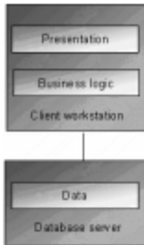
Figure 1.6 Two-tier (fat client) architecture
